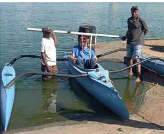
Using a sling on a boom to lift Alwyn into his boat.
